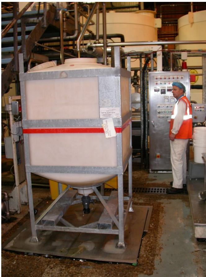
MTV 1000 fitted with fork tunnels
